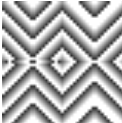
Figure 13: Spiral wave in the excitable automata model [5]. There are six states, 0 through 5. If any cell is at state 5 it is set to state 0 (resting). Any other excited or refractory (i.e., nonzero) state is incremented by 1. If a cell is resting and one of its four neighbors is excited (state 1), then the cell becomes excited, otherwise it remains at rest. White corresponds to state 0 and black to state 5.
