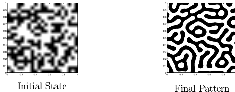
Figure 14: Isotropic pattern formation after 100 steps starting from a random checkerboard pattern. In this case, the kernel consists of the difference of two Gaussian distributions: K(x, y) = \frac{2500}{\pi} \exp(-2500|\vec{x}|^2) - \frac{1250}{3\pi} \exp\left(-\frac{1250}{3}|\vec{x}|^2\right) .
